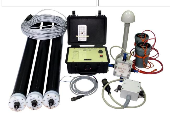
Wide band magnetotelluric station LEMI-423 is intended for the study of natural electromagnetic fluctuations in field conditions in wide temperature range. The station registers and digitizes automatically the data from 3 search-coil magnetometers and 2 electric channels and monitors the temperature of electronic unit. The electric channels include lightning protection unit,
