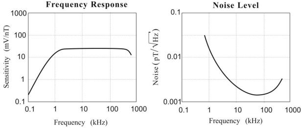
New calculation methodology using minimal mass criterion allowed minimizing the weight, conserving low noise level in wide frequency band. The magnetic feedback design is utilised what provides a stable response of full frequency band. Low noise preamplifier is placed inside the sensor body.
