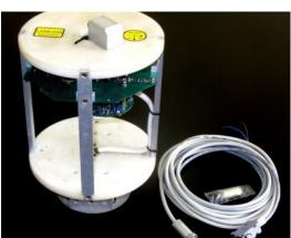
needs of fundamental and applied geophysics. It has no external housing being destined for the installation inside sealed housing of sea bed station (see photo on the left). Because of this any customization of dimensions are possible at the customer's request. It has two-component tiltmeter and does not contain GPS receiver and nonvolatile memory. For data registration it has to be coupled with a basic station by a cable
