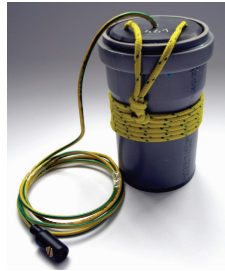
Figure 1: LEMI-701 ultra-low noise non-polarized electrodes.
