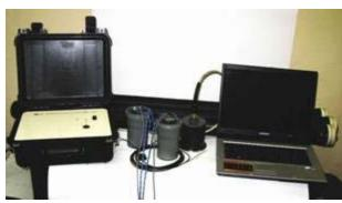
Earth's crust electromagnetic structure in frequency band (DC-200) Hz in field conditions in wide temperature range. The station maintains automatically measurements and digitizing data from the flux-gate and search-coil magnetometers, 4 telluric channels and temperatures of sensor and electronics. The real time acquisition, recording and
