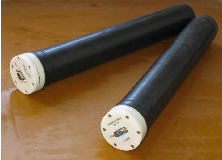
LEMI-121 Induction Magnetometers
